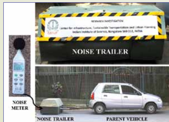
Figure 2. Field Tyre / Pavement Noise Measurement Equipment Setup
