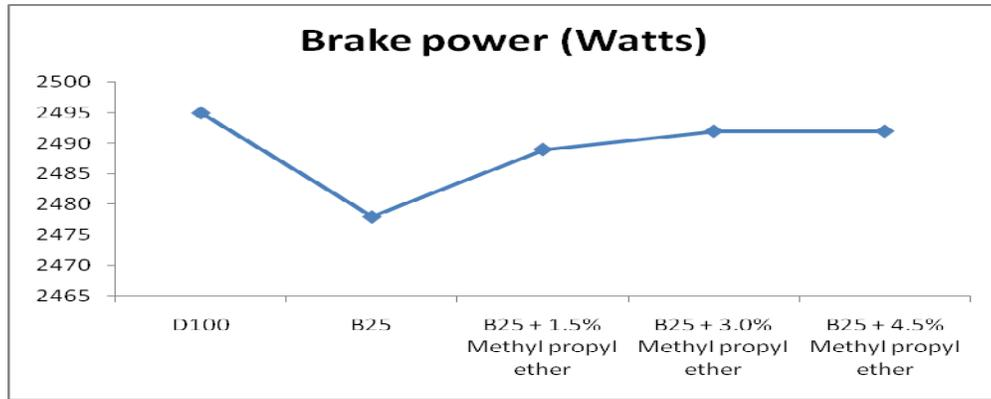
Figure 35. Power output with Methyl Propyl Ether with blends
