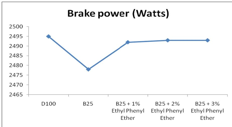
Figure 30. Comparison of break Power output with Phenyl ethyl ether blends
