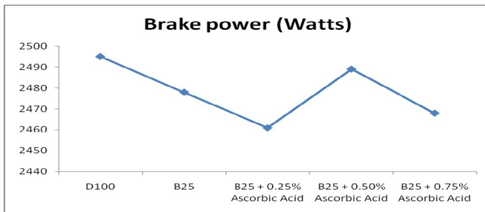
Figure 20. Comparison of Break Power output with Ascorbic Acid blends
