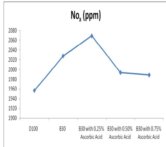
Figure 18. Variation of CO<sub>2</sub> emissions with Ascorbic acid blends Figure 19. Variation of NO<sub>x</sub> emissions with Ascorbic acid blends
