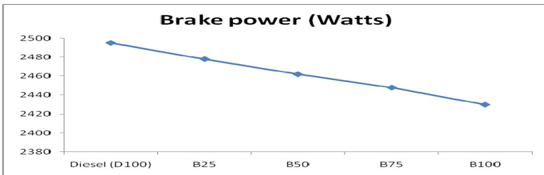
Figure 11. Comparison of Break Power output with various fuel blends
