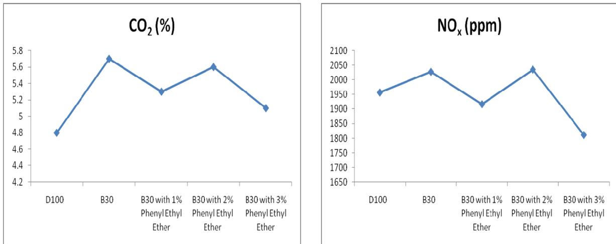
Figure 28. variation of CO<sub>2</sub> emissions with Phenyl ethyl ether blends Figure 29. Variation of NO<sub>x</sub> emissions with Phenyl ethyl ether blends
