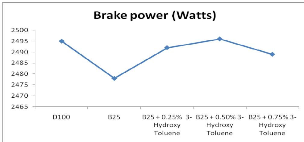
Figure 25. Power output with 3- Hydroxy Toluene
