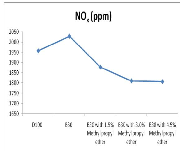
Figure 33. Variation of CO<sub>2</sub> emissions with methyl propyl ether blends Figure 34. Variation of NO<sub>x</sub> emissions with methyl propyl ether blends
