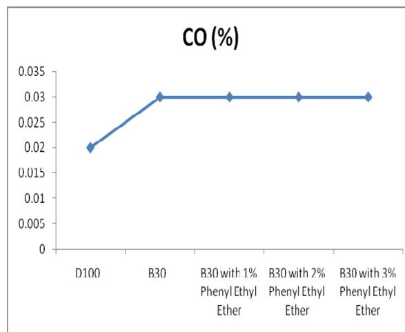
Figure 26. Variation of HC emissions with Phenyl ethyl ether blends Figure 27. Variation of CO emissions with Phenyl ethyl ether blends
