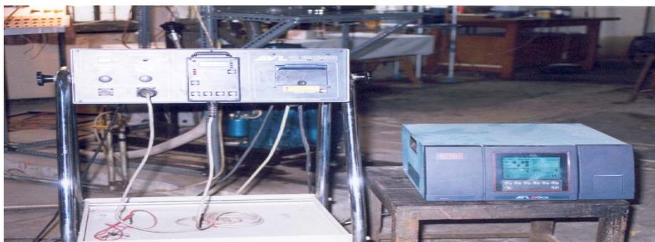
Figure.9 Five Gas Emission Analyzer
