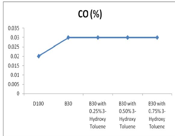
Figure 21. Variation of HC emissions with 3-hydroxy toluene blends Figure 22. Variation of CO emissions with 3-hydroxy toluene blends
