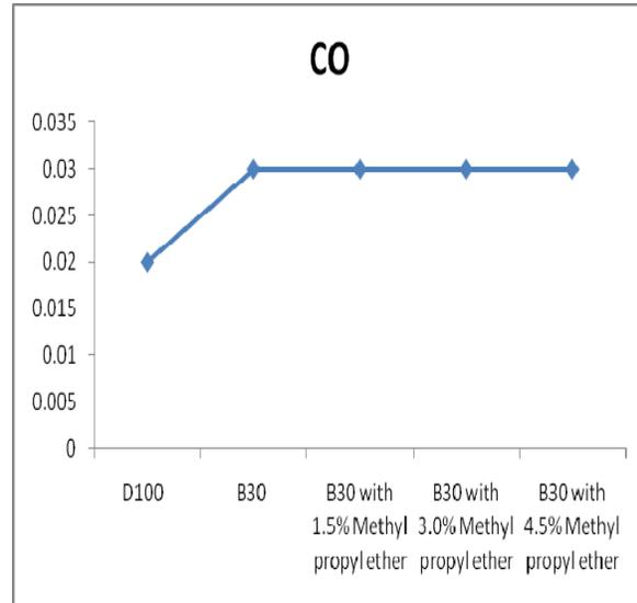
Figure 31. Variation of HC emissions with methyl propyl ether blends Figure 32. Variation of CO emissions with methyl propyl ether blends
