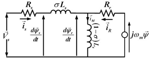
Fig. 1 Space Phasor based equivalent circuit of induction motor with rotor flux as a reference vector
