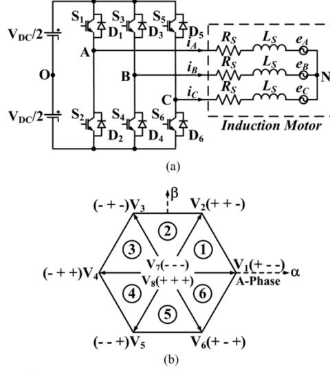
Fig. 2 (a) Power schematic of a three-phase two-level Voltage Source Inverter (VSI) fed induction motor drive, and (b) Voltage space phasor structure of the two-level voltage source inverter
