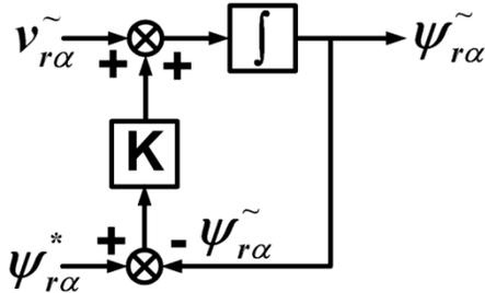
Fig. 3 Block diagram for realization of integration of calculated rotor voltage for estimation of rotor flux.
